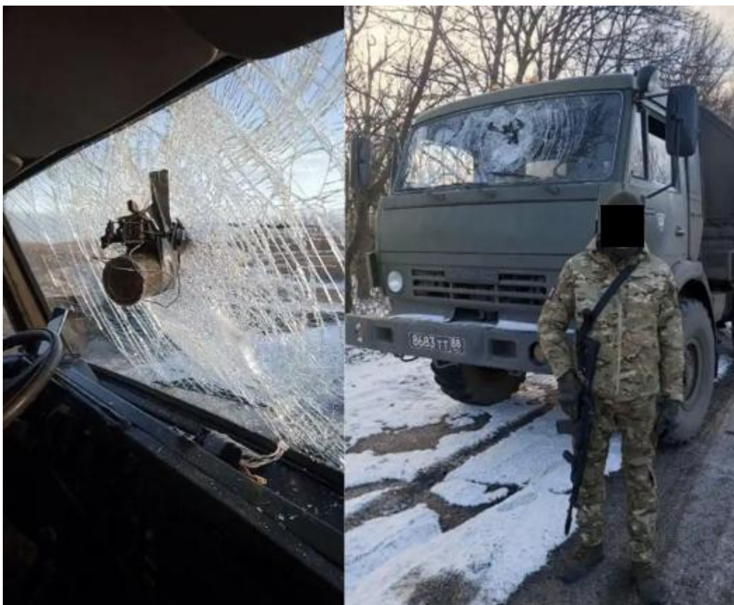
OWA UAV Quadcopter failed to detonate of impact into Russian vehicle's windshield.
