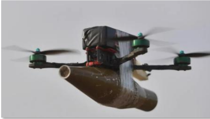
Russian drone Modified with rocket warhead.
